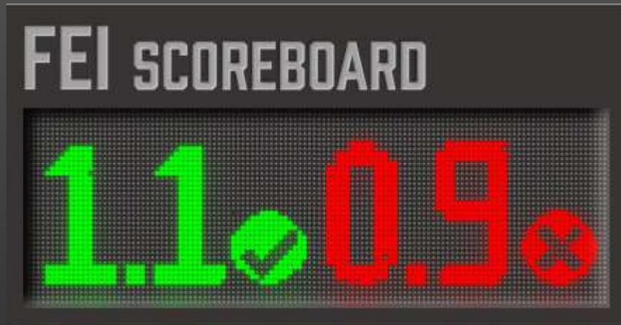
$$FEI = \frac{\text{Reference Fan Electrical Input Power}}{\text{Actual Fan Electrical Input Power}}$$
